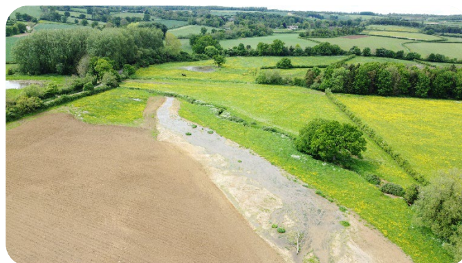
Drone-view of the brook, with water diverted across land, away from the deep-cut channel.
