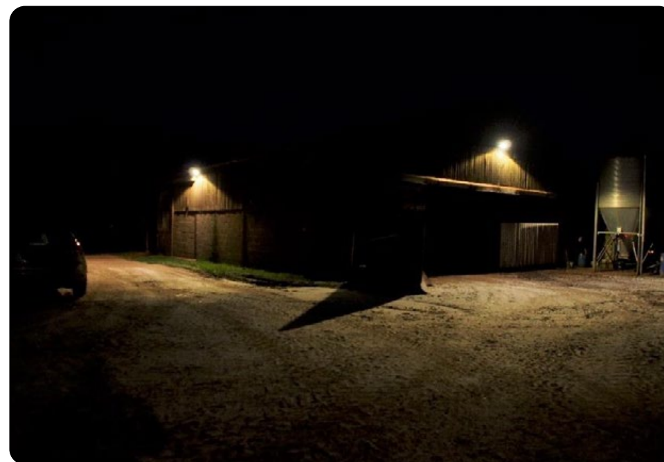
Figure 16 – An example of good farm lighting. Courtesy Mike Hawtin. North York Moors National Park. Note the correct colour temperature, direction, shielding and appropriate levels of illuminance for safe working.
